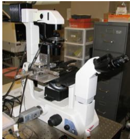
Figure 8: Experimental setup 1, tuning fork, oscillating fiber, microscopy and video/image taking system. 2, Photron APX RS high speed camera. 3, Nikon TE200 inverted fluorescence microscopy.
